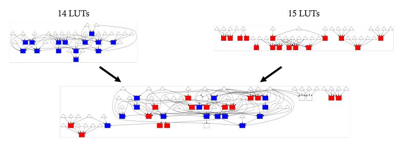
Initial mapping to LUT Subgraph extraction Iterative area minimization Recombine subgraphs
