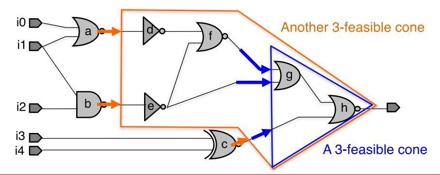
Delay estimation in HLS is inaccurate without considering LUT mapping
