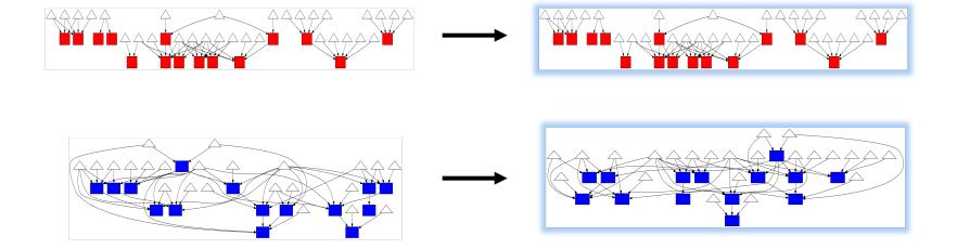
Initial mapping to LUT Subgraph extraction Iterative area minimization Recombine subgraphs
